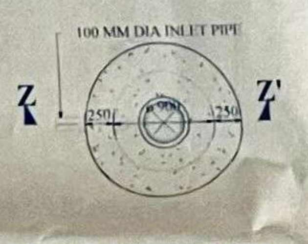
DETAIL OF SOAK PIT SCALE - 1 : 50
